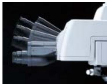
The eyepiece tube is of the trinocular tilting type, allowing continuous adjustment of the tilt angle from 0° to 30° for viewing at the optimum eyepoint level. The eyepiece also features an ultrawidefield design and has an F.O.V. of 25mm.
