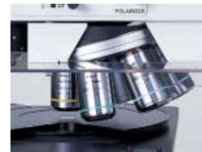
The built-in nosepiece is a motorized sextuple type with a slot for DIC attachment. In addition to a mechanical click stop, this nosepiece is controlled by software to stop precisely at each objective position. The improved accuracy also dramatically increases the durability of the nosepiece. Moreover, when the nosepiece is rotated, the illumination is cut momentarily to protect the operator's eyes.
